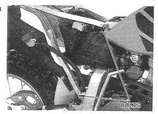
Install the upper chain slider and tighten the left lower sub-frame mounting bolt.
