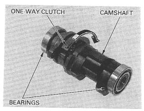
Remove the bearings from the camshaft. Check each cam lobe for wear or damage.
