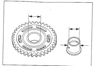
Measure the O.D. of the countershaft at the idle gear bushing sliding surface.
