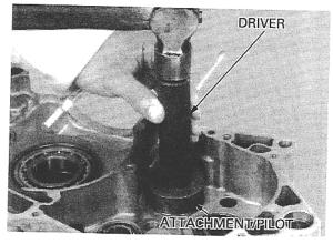
bearings squarely special tools. with the marking side facing toward TOOLS: the inside of the Driver
