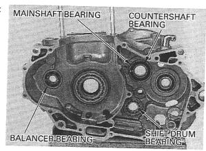
bearings squarely with the marking side facing toward TOOLS: the inside of the Driver
