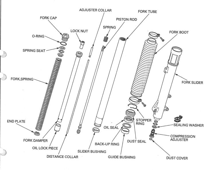
Install the oil seal with its marked side facing the dust seal. Install the following from the fork tube upper side:
