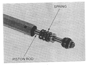
Install the lock nut to the damper rod.
