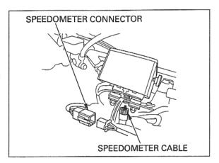
Remove the two nuts and speedometer.
