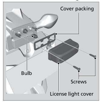
**3.** Install a new bulb and parts in the reverse order of removal.
