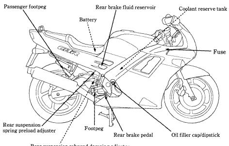
Rear suspension rebound damping adjuster
