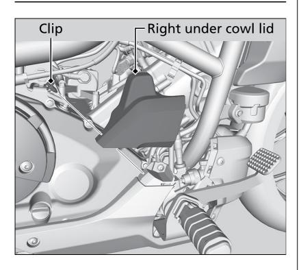
The right under cowl lid must be removed to service the coolant reserve tank and brake light switch.
