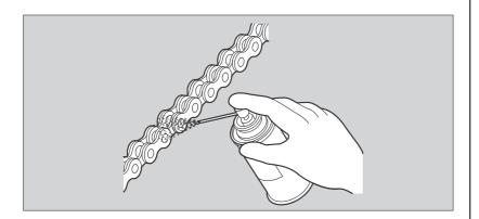
Never use petrol or low flash point solvents for cleaning the drive chain. A fire or explosion could result.
