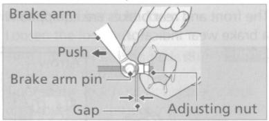
After adjustment, confirm the freeplay of the brake lever.
