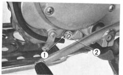
Tensioner adjusting bolt lock nut
