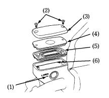
Brake fluid must be added to the reservoir whenever the fluid level begins to reach the LOWER level mark (1). Remove the screws (2), reservoir cover (3), diaphragm plate (4), and diaphragm (5). Fill the reservoir with DOT 4 BRAKE FLUID from a sealed container up to the upper level mark (6). Reinstall the diaphragm, diaphragm plate, and cover. Tighten the screws securely.
