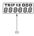
(1) Odometer/tripmeter/digital clock display
