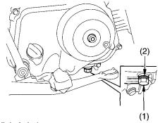
(1) oil drain bolt(2) sealing washer
