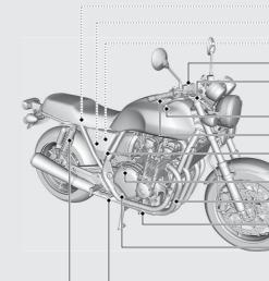
Rear brake fluid reservoir Battery P.61 Air cleaner Front brake fluid reservoir P.74 Front suspension spring preload adjuster P.88 Front brake lever P.87 Throttle grip P.84 Right side cover C>P.65 Engine oil fill cap P.68 Engine oil filter P.70 Engine oil drain bolt P.70 Engine oil level inspection window ►P.68 Rear brake pedal
