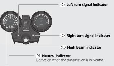
Comes on briefly when the ignition switch is turned to the ON position with the engine stop switch in the  $\bigcirc$  (Run) position.
