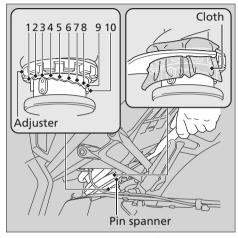
Attempting to adjust directly from 1 to 10 or 10 to 1 may damage the shock absorber.
