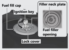
Do not fill with fuel above the filler neck plate. **Fuel type:** Unleaded gasoline only **Recommended fuel octane number:** Pump Octane Number (PON) 86 or higher.
