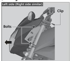
1. Remove the bolts and clip (▶ P. 53) on both sides and pull the headlight assembly forward.
