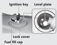
Do not fill with fuel above the level plate. Fuel type: Unleaded gasoline only Recommended fuel octane number: Pump Octane Number (PON) 86 or higher. Tank capacity: 4.41 US gal (16.7 L)
