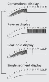
2 Press SET button. The currently selected displaying mode is set, and the control returns to the ordinary display.
