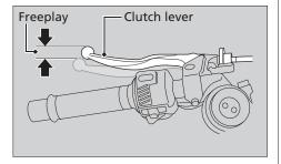
Check the clutch cable for kinks or signs of wear. If necessary have it replaced by your dealer.
