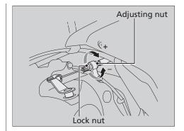
If proper adjustment cannot be obtained or the clutch does not work correctly, see your dealer.
