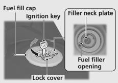
Do not fill with fuel above the filler neck plate. **Fuel type:** Unleaded gasoline only **Recommended fuel octane number:** Pump Octane Number (PON) 86 or higher. **Tank capacity:** 3.43 US gal (13.0 liters)
