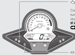
PGM-FI (Programmed Fuel Injection) malfunction indicator lamp (MIL)
