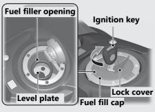
Do not fill with fuel above the level plate. **Fuel type:** Unleaded gasoline only **Recommended fuel octane number:** Pump Octane Number (PON) 86 or higher. **Tank capacity:** 4.07 US gal (15.4 L)
