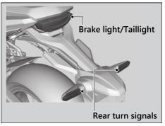
The brake light and taillight use several LEDs. Each right and left rear turn signal uses an LED.
