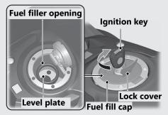
Do not fill with fuel above the level plate. **Fuel type:** Unleaded gasoline only **Recommended fuel octane number:** Pump Octane Number (PON) 86 or higher. **Tank capacity:** 4.07 US gal (15.4 L)
