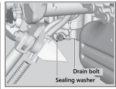
Remove the oil fill cap/dipstick, drain bolt, and sealing washer to drain the oil.
