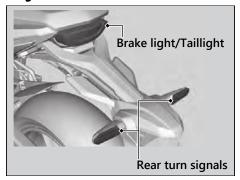
The brake light and taillight use several LEDs. The rear turn signals uses an LED.
