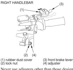
Never use adjusters other than those designed for this motorcycle. Install a new adjuster from the lever side with the lock nut under the head of the adjuster.
