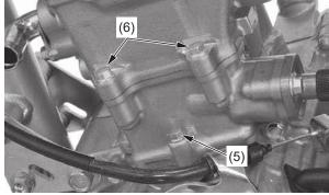
(5) cylinder bolt(6) cylinder head bolts
