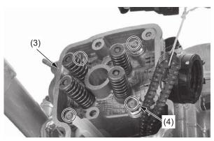
(3) cylinder head(4) cylinder head nuts/washers
