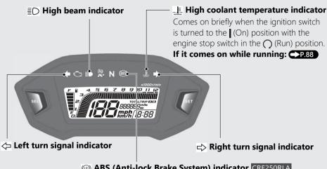
(S) ABS (Anti-lock Brake System) indicator CRF250RLA Comes on when the ignition switch is turned to the (On) position. Goes off when your speed reaches approximately 6 mph (10 km/h). If it comes on while riding: →P.89
