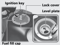
Do not fill with fuel above the level plate. **Fuel type:** Unleaded gasoline only **Recommended fuel octane number:** Pump Octane Number (PON) 86 or higher. **Tank capacity:** 2.67 US gal (10.1 L)
