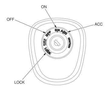
The ignition switch is used for starting and stopping the engine (page 53) and to lock the steering for theft prevention (page 63). Insert the key and turn it to the right for the ON and ACC (accessory) positions.
