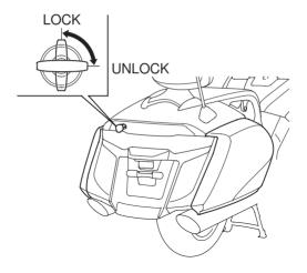
The saddlebags can be locked and unlocked with the ignition key.
