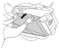
To shut the saddlebags, place your hands flat on the edges of its lid and press down until it is firmly closed and check the saddlebags open indicator is not displayed.
