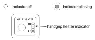
When you are making a temporary stop or riding at low speed, the battery voltage level may go down. This can turn off the handgrip heater automatically. The heater then resumes it operation when the battery voltage level recovers after riding for a while.
