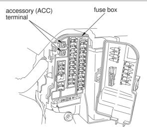
For your convenience, your motorcycle is equipped with an accessory (ACC) terminal and optional accessory socket. The terminal and socket provide 12V DC power for electrical accessories. When both terminal and socket are being used, the combined power rating of each accessory should be 60 watts (5 amps) or less. Before installing any accessories, read *Accessories and Modifications*, page 4.
