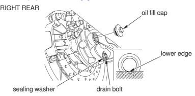
Change the oil with the final drive at normal operating temperature to assure complete and rapid draining.
