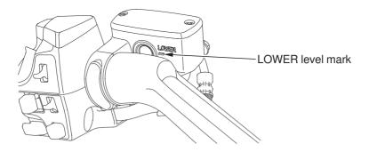
Check that the fluid level is above the LOWER level mark. If the fluid level is below the LOWER level mark, it indicates fluid leakage. See your dealer for repair.
