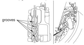
Always inspect both pads in both the right and left front brake calipers.
