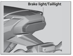
The brake light and taillight uses several LEDs. If there is an LED which is not turned on, see your dealer for servicing.
