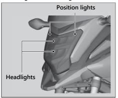
The headlights and position lights uses several LEDs.
