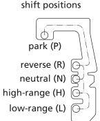
You should move the shift select lever only when the vehicle is stopped with your foot on the brake pedal and with the engine idling. Use a firm motion to select the appropriate gear. Have your vehicle checked by a dealer if you experience any shifting problems.
