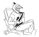
To unlatch a seat belt, press the red PUSH button on the buckles.
