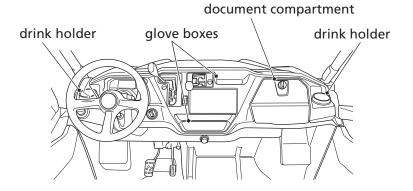
To open the document compartment, turn the knob clockwise. To close the document compartment, turn the knob counterclockwise.
