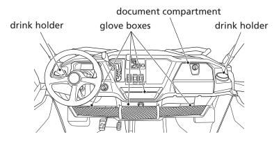
To open the document compartment, turn the knob clockwise. To close the document compartment, turn the knob counterclockwise.
