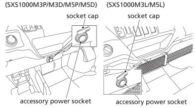
To use the accessory power socket, the engine must be running.
